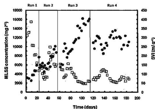
Fig. 5 Profiles of MLSS level and SVI value of sludge in the SB reactor: (●) MLSS; (□) SVI.
