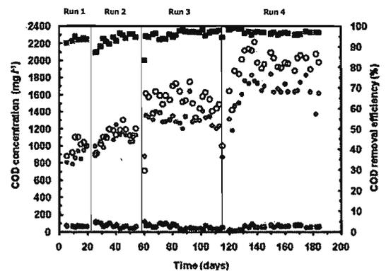
Fig. 3 Changes in COD removal performance: (■) COD removal efficiency; (○) influent COD; (⊙) AF effluent COD; (●) final effluent COD.
