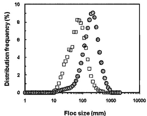
Fig. 7 Floc size distribution of sludge in the SB reactor: (□) Seed sludge, mean size:  $76 \mu\text{m}$ ; (●) Run 4, day 149, mean size:  $213 \mu\text{m}$ .
