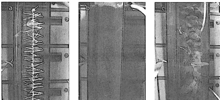
Fig. 8 Photograph of biofilm attached the BF carrier: (a) vacant reactor; (b) running state in Run 3; (c) attached biofilm after suspended sludge removal at the end of Run 3.
