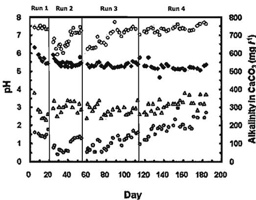
Fig. 2 Profiles of pH and alkalinity in AF and final effluents: (◆) AF effluent pH; (○) final effluent pH; (△) AF effluent alkalinity; (⊙) final effluent alkalinity.
