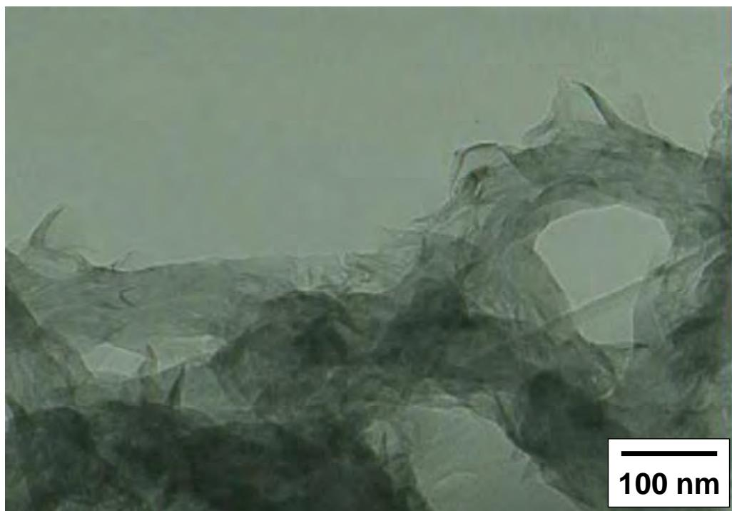
**Fig. 3.7** TEM image of the products on the surface of a ceramic heater for synthesis temperature of 1000 °C. Fe nanoparticles embedded in zeolites are attached in the center of the heater. Observed fibriform materials with a diameter of about 70-80 nm are distorted.
