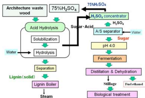
Fig. 10 Block diagram for production of fuel ethanol from cellulose biomass
