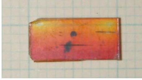
Fig. 1. A photograph of a  $\text{Cu}_2\text{O}$  thin film sandwiched by MgO plates. The dimensions of the sample are  $5 \times 10 \times 1 \text{ mm}^3$ . The thickness of the  $\text{Cu}_2\text{O}$  thin film is  $1.3 \sim 4.3 \text{ }\mu\text{m}$ .<sup>5)</sup>
