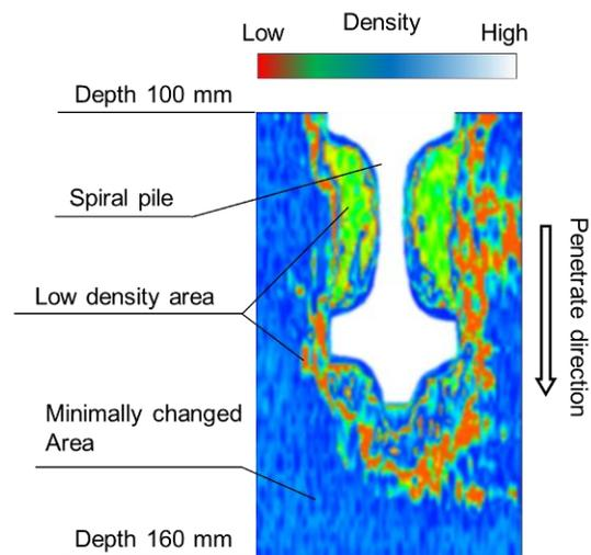
Figure 5: Vertical cross-sectional CT image (free rotate penetration)
