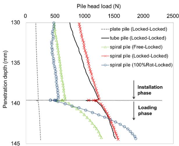
Figure 4: Relationship between pile head load and penetration depth
