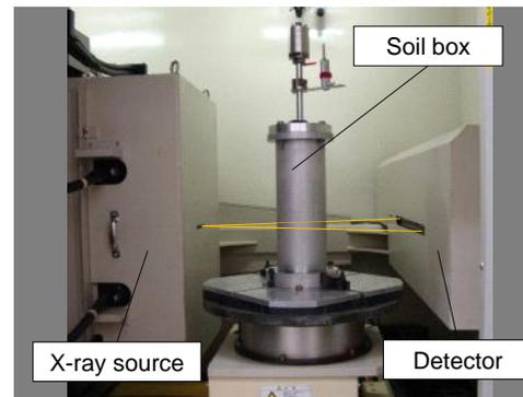
Figure 3: State of X-ray CT scanning
