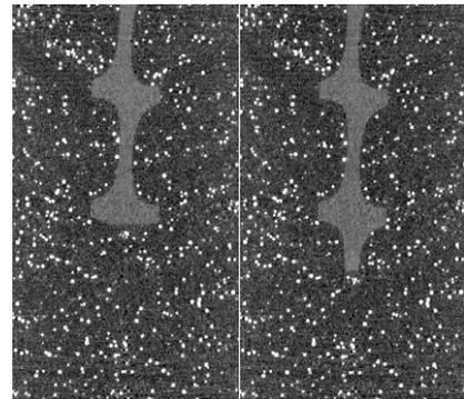
Figure 7: Observation of particle displacement on stepwise pile penetration test using Micro-focus X-ray CT image
