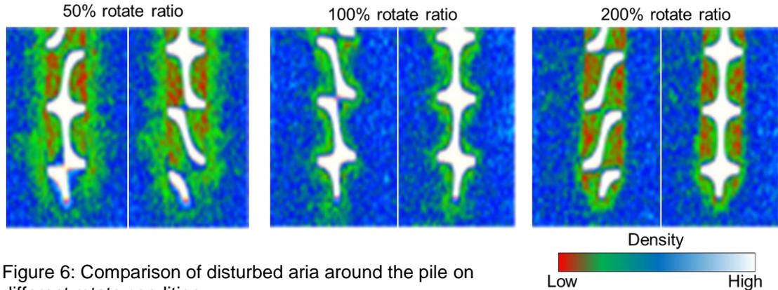
Figure 6: Comparison of disturbed area around the pile on different rotate condition
