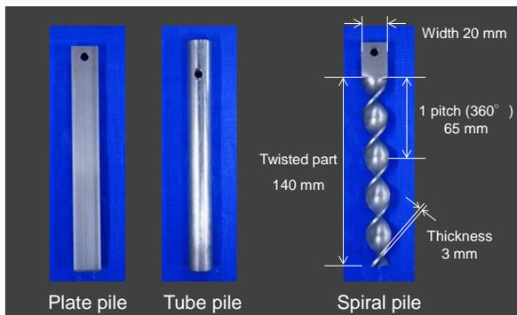
Figure 1: Model piles and details of spiral pile
