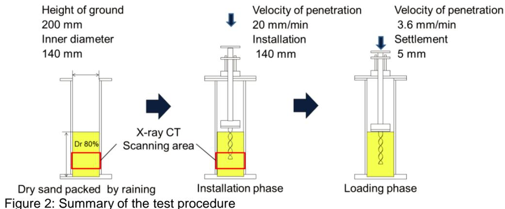
Figure 2: Summary of the test procedure
