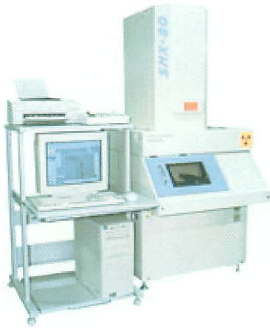
Fig. 3-1 Photograph of micro focus X-ray TV system.
