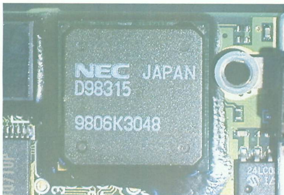
Fig. 3-12 Photograph of BGA on board.
