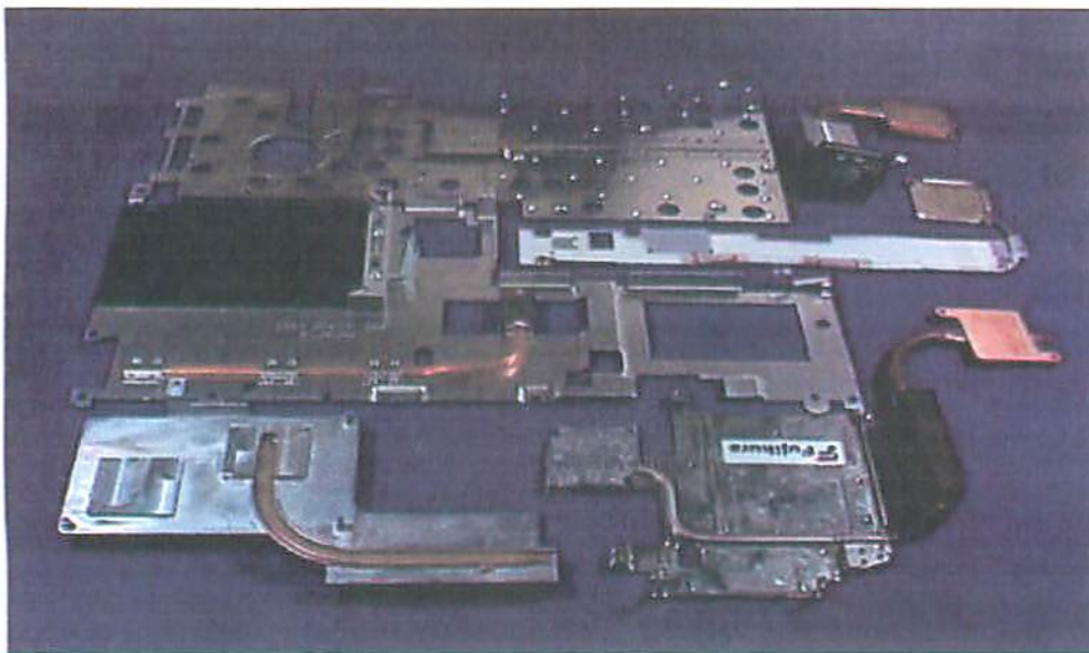
Fig. 6-4 Various real products of passive cooling part consisting of heat spreader with heat pipe
