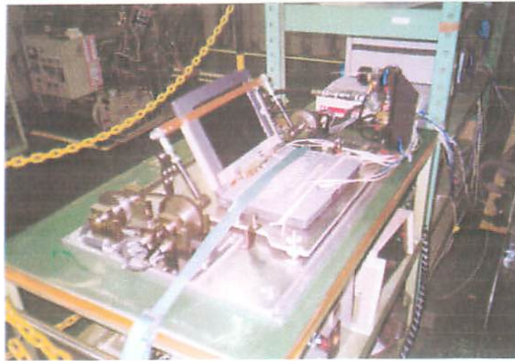
Fig. 6-9 Reliability test equipment of thermal hinge heat pipe
