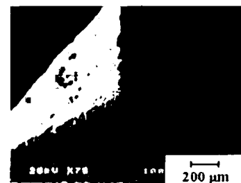
Figure 4.2. Typical SEM image of the top of a \beta''\text{-Al}_2\text{O}_3 microelectrode.
