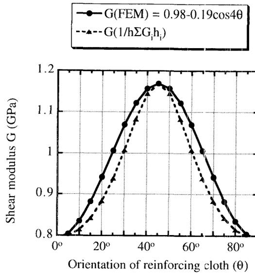
Fig. 5. Relationship between shear modulus and orientation of reinforcing cloth.
