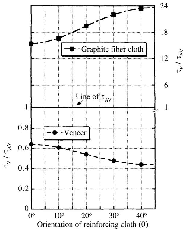
Fig. 6. Comparison of shearing stress among different reinforced plywoods.
