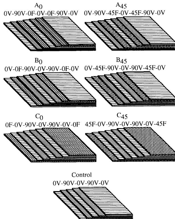
Fig. 3. Seven types of graphite fiber reinforced plywoods.
