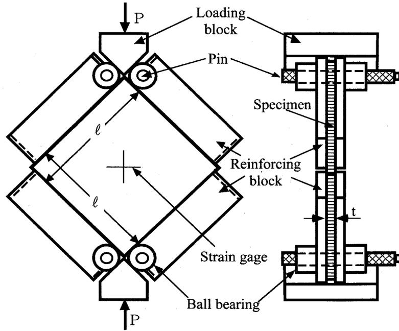
Fig. 1 Apparatus and method of panel shear testing (ASTM).
