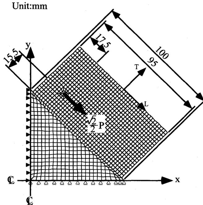
Fig. 3 Analytical model for finite element method.
