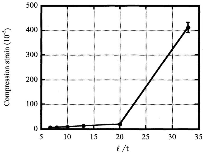
Fig. 8 Average compression strains versus length thickness ratio of specimen.
