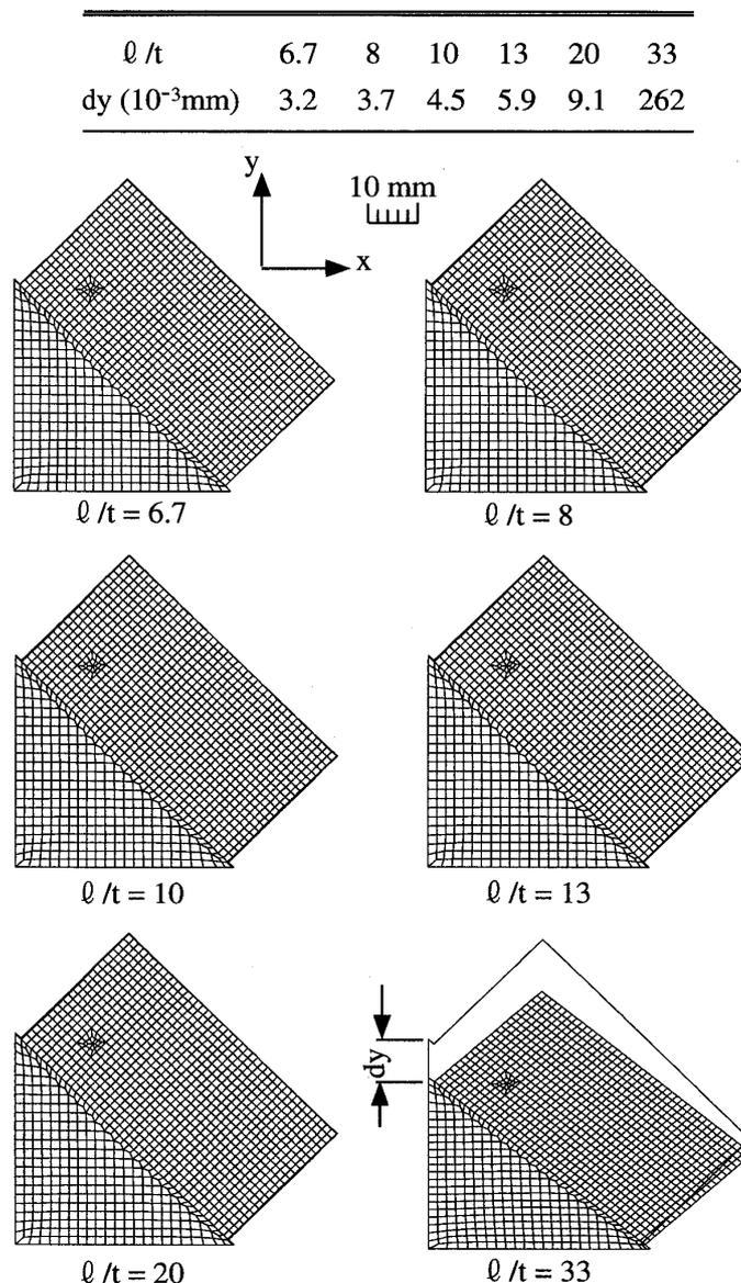
Fig. 4 Deformations of the specimens with different length thickness ratios ( $l/t$ ). Note: Values of the displacement are expressed in magnification,  $\times 50$ .
