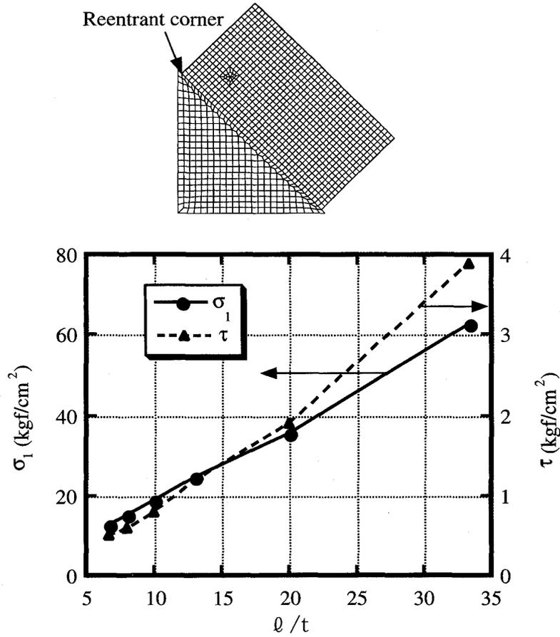
Fig. 7 Maximum principal stress  $\sigma_1$  and  $\tau$  at the reentrant corner of the specimens.
