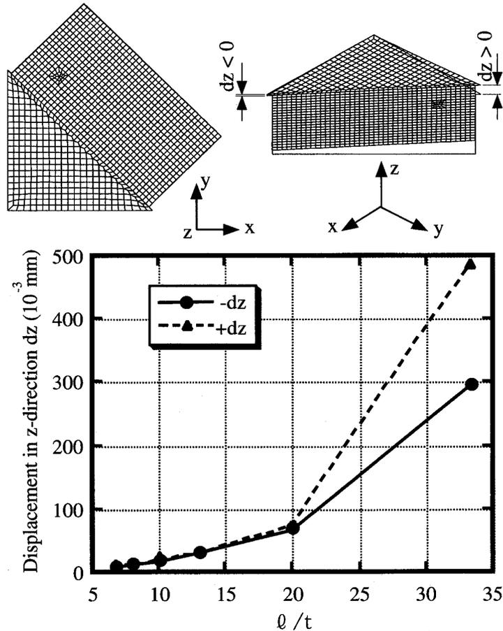
Fig. 5 Maximum displacements in z-direction.
