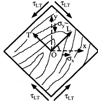
Fig. 2 Diagram used to calculate stress and strain in panel shear of plywood with face grain parallel to edge.
