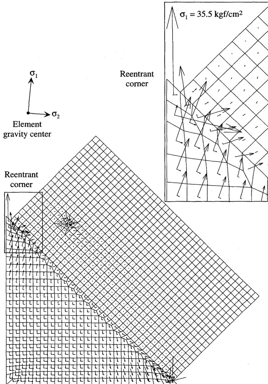
Fig. 6 Distribution of principal stresses  $\sigma_1$  and  $\sigma_2$  in specimen with length thickness ratio of 20.
