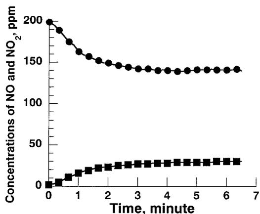
Fig. 6. Dependence of NO and NO<sub>2</sub> concentrations on time of application of pulsed power. Pulse rate: 1 pps; pulselength: 120 ns. Other conditions are as in Fig. 4. ● NO, ■ NO<sub>2</sub>.
