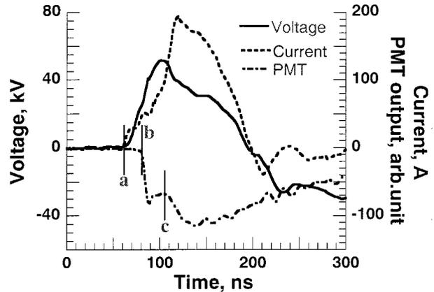
Fig. 9. Applied voltage, discharge current, and photo multiplier tube (PMT) current as a function of time during the application of a single power pulse to the coaxial reactor. Times  $a$  to  $c$  are defined in the text. Nominal pulsewidth, 100 ns; other conditions are as in Fig. 4.
