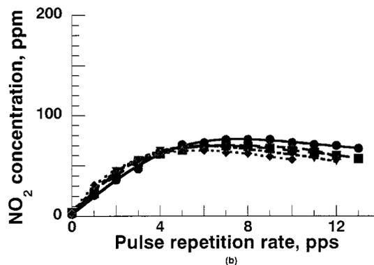
Fig. 7. Final concentrations of nitric oxide (a) NO<sub>f</sub> and (b) NO<sub>2</sub> as a function of pulse repetition rate for different pulsewidths. Other conditions are as in Fig. 4. ● 40 ns, ■ 60 ns, ◆ 80 ns, ▲ 100 ns, and ▼ 120 ns.
