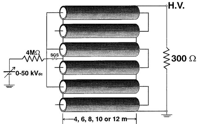
Fig. 1. Three-stage Blumlein generator showing the charging voltage (0–50 kV), the charging resistance (4 M $\Omega$ ), the spark gap switch (SGS), and the matching output resistance (300  $\Omega$ ). The cable length varied from 4–12 m giving pulsewidths of 40, 60, 80, 100, and 120 ns. Three hundred ohms was removed when coaxial reactor was used.
