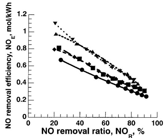
Fig. 14. Dependence of the energy efficiency of the removal of NO ( $\text{NO}_E$ ) on the removal ratio or NO for different discharge currents. Pulsewidth, 100 ns; other conditions are as in Fig. 4. • 0  $\Omega$  (185 A), ■ 50  $\Omega$  (156 A), ◆ 100  $\Omega$  (137 A), ▲ 200  $\Omega$  (114 A), and ▼ 300  $\Omega$  (98 A).
