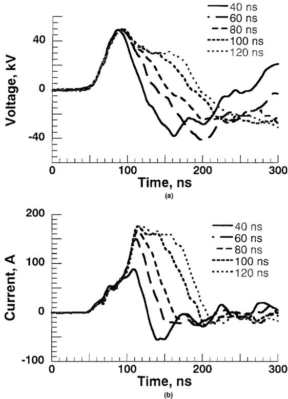
Fig. 4. (a) Applied voltage to and (b) discharge current in the coaxial reactor for varying pulsewidths. Conditions: gas pressure:  $1.01 \times 10^5$  Pa; NO: 200 ppm; O<sub>2</sub>: 5%; H<sub>2</sub>O: 4%, and balance N<sub>2</sub> gas flow rate: 2.0 l/min; series resistance with reactor, 0  $\Omega$ . Parallel resistance was disconnected.
