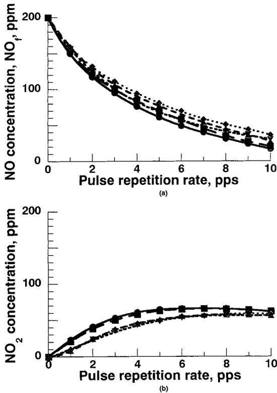
Fig. 13. Final concentrations of nitric oxide, (a)  $\text{NO}_f$  and (b)  $\text{NO}_2$  as a function of the pulse repetition rate for different series resistances (and peak currents) with the coaxial reactor. Nominal pulsewidth, 100 ns; other conditions are as in Fig. 4. • 0  $\Omega$  (185 A), ■ 50  $\Omega$  (156 A), ◆ 100  $\Omega$  (137 A), ▲ 200  $\Omega$  (114 A), and ▼ 300  $\Omega$  (98 A).
