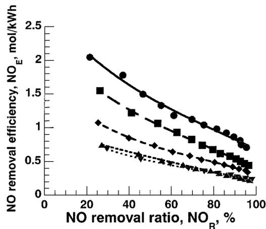
Fig. 8. Dependence of the energy efficiency of the removal of NO (mol/kWh) on the removal ratio of NO<sub>R</sub> (%). Other conditions are as in Fig. 4. ● 40 ns, ■ 60 ns, ◆ 80 ns, ▲ 100 ns, and ▼ 120 ns.
