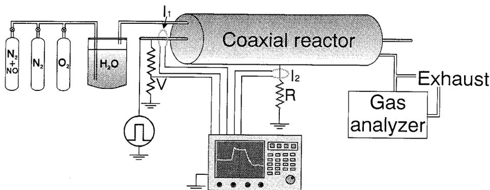
Fig. 2. Experimental set-up for removal of NO using a concentric electrodes reactor:  $I_1$ : current into the reactor;  $I_2$ , current in the external resistance  $R$ ; value of  $R$ : 0, 50, 100, 200, and 300  $\Omega$ . Resistance divider, 1  $\Omega/5$  k $\Omega$ .
