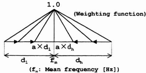
the base is a function of the mean frequency, as in Fig. 4(b). This triangular weighting function is effective to remove reasonably zero-crossing intervals disturbed by influence of sound source, which are far from the center of the distribution. When a set of zero-crossing frequencies is given as  $\{f_i\}$  in  $i = 1, 2, \dots, M$ , a weighted mean  $\bar{f}_m$  is computed using the weighting function  $W(f_m; f)$  as
