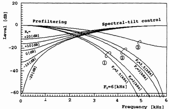
Fig. 3. Characteristics of prefiltering and spectral-tilt control.
