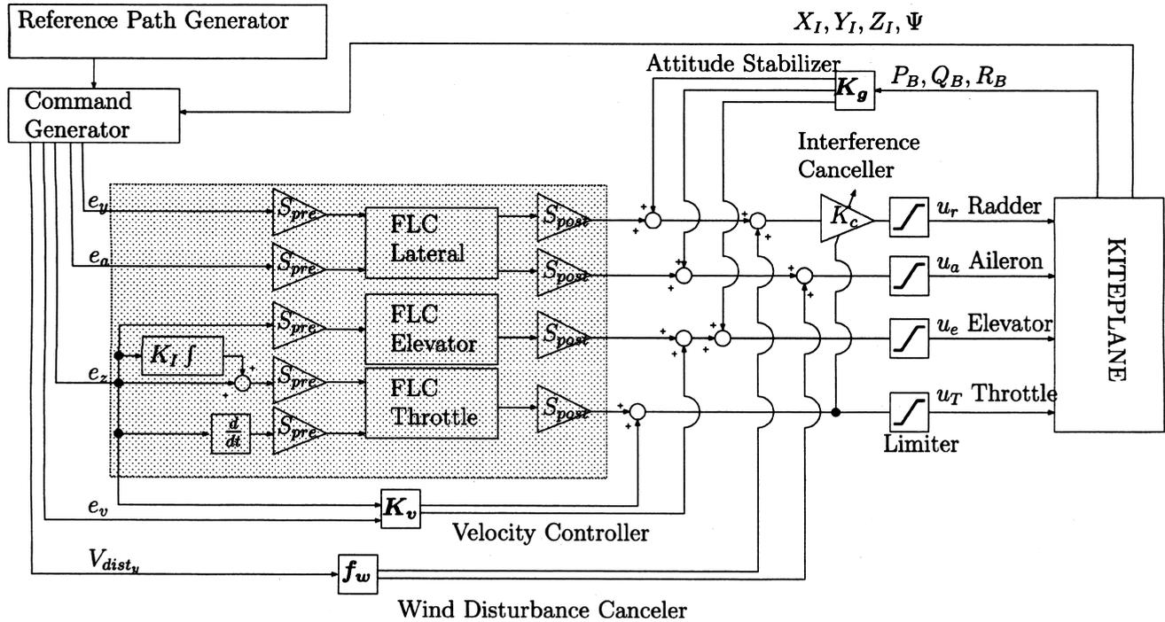
Fig. 6. Block diagram of the autopilot system.
