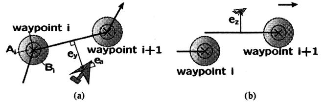
Fig. 4. Reference path. (a) Lateral reference. (b) Longitudinal reference.
