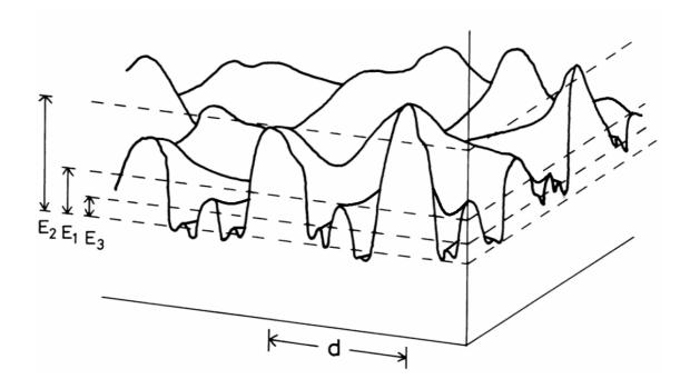
**Fig. 1.** A schematic representation of the energy barrier profile in superionic glasses.  $E_1$  and  $E_2$  are the average values of the activation energies in the doped salt and in the network, respectively.  $E_3$  is the activation energy of the highly conducting region. d is a characteristic distance that defines the medium range structure.
