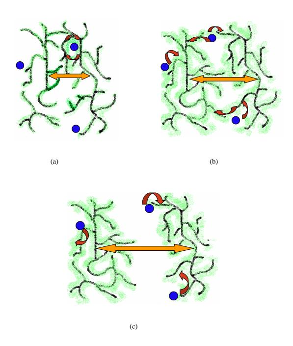
Fig. 4. A schematic representation showing how the connectivity of the highly conducting regions, or the low activation energy sites (illustrated as spreads around the network skeleton) vary with the concentration of doped salts (not explicitly shown for clearness). The doped salt concentration increases from (a) to (c) and expands the network separation.
