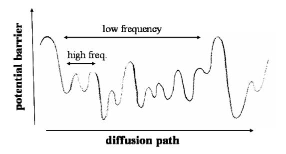
**Fig. 2.** At low frequencies, the mobile ion explores a large space in the potential barrier profile, whereas at high frequencies, it explores a local barrier profile.
