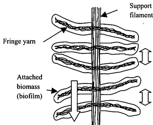
Fig. 4- 2 Configuration for biomass carrier
