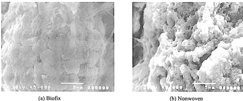
Fig. 3- 7 Comparison of surface condition of granular sludge
