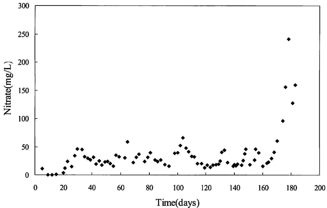
Fig. 4- 8 Time course of effluent nitrate concentrations in PN reactor
