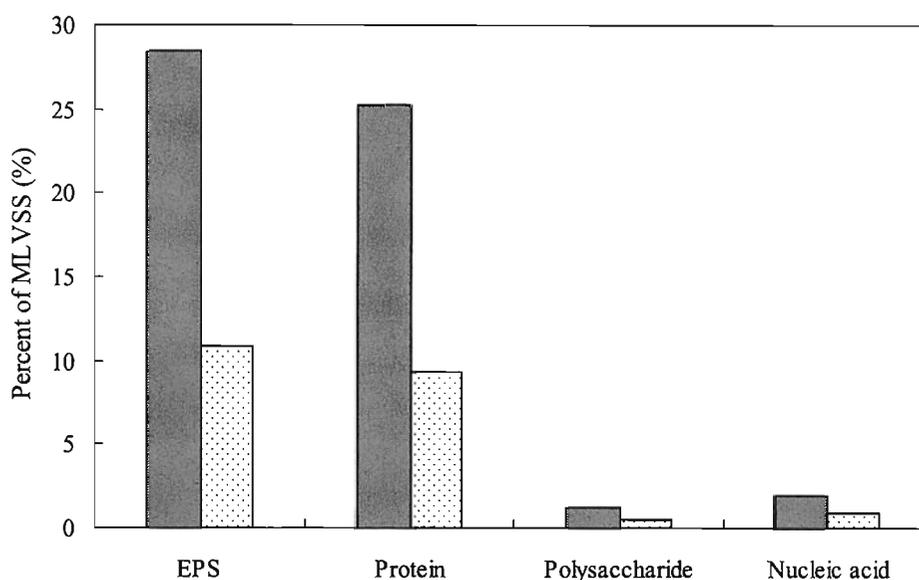
Fig. 3- 6 EPS comparison of granular sludge in Biofix and nonwoven reactor
