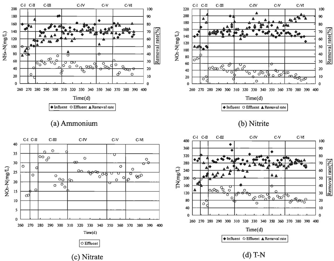
Fig. 2-6 Time courses of nitrogen concentrations during phase C
