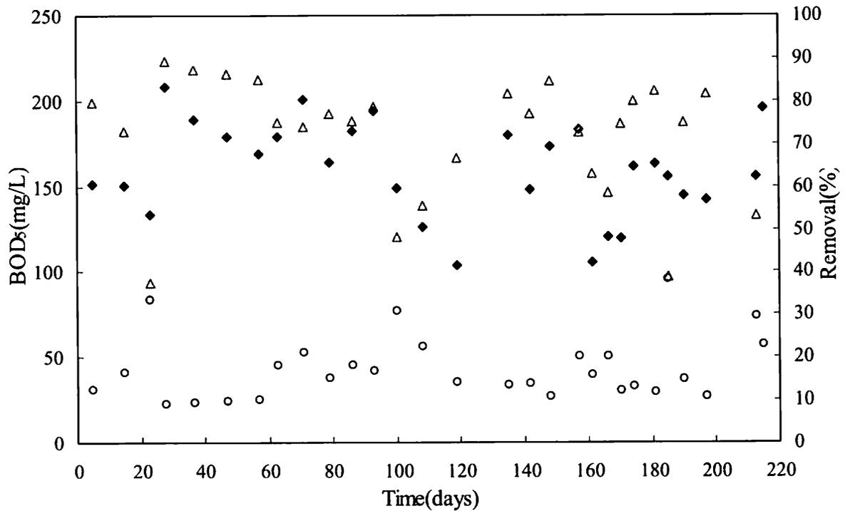
Fig. 4- 4 Time courses of BOD<sub>5</sub> removal performances in PN reactor
