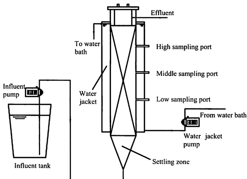
Fig. 2- 1 Schematic diagram of the up-flow anammox column reactor
