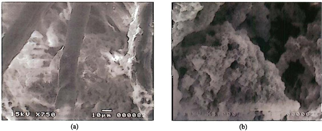
Fig. 2- 9 SEM of anammox sludge attached on Biofill
