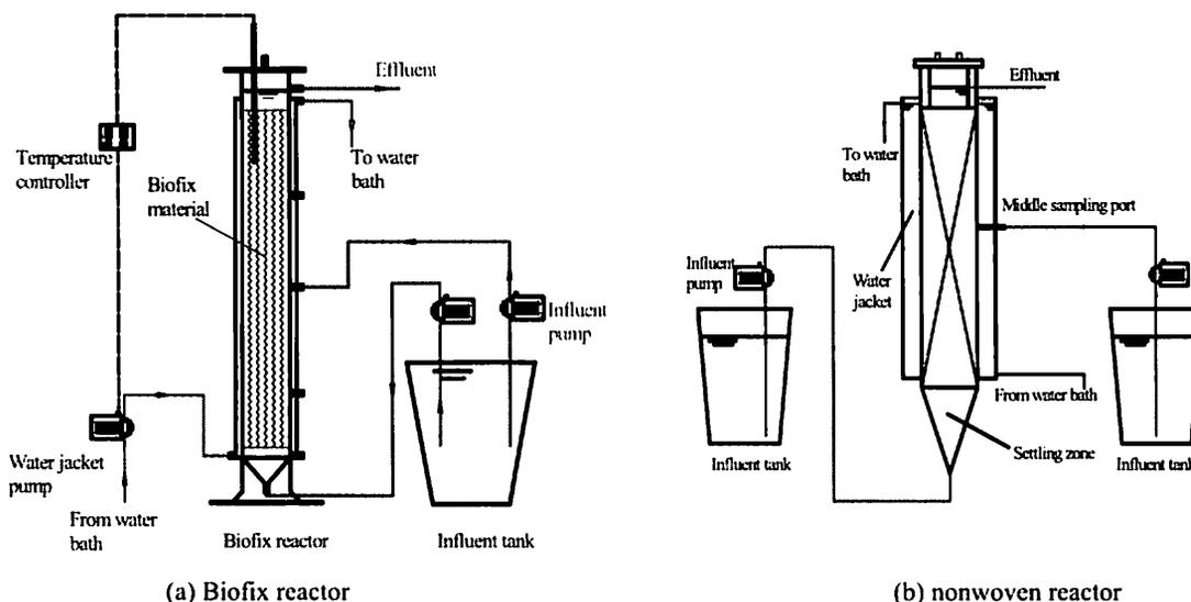
Fig. 3- 1 Schematic diagram of Biofix and nonwoven reactors
