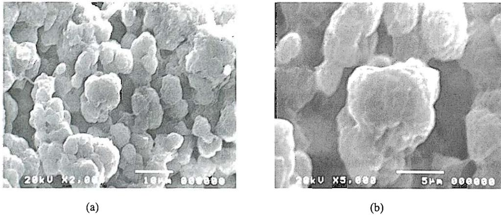
Fig. 3- 8 SEM photos of attached biomass on Biofix
