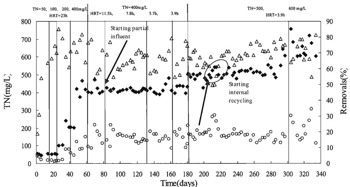
Fig. 3- 2 Time courses of T-N concentration and removal rates
