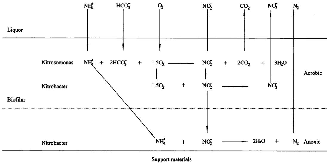
Fig. 1- 5 Synergetic model of nitrification and denitrification
