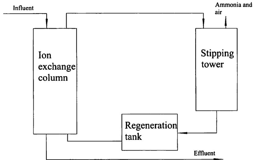
Fig. 1- 3 Selective ion exchange process for ammonia removal
