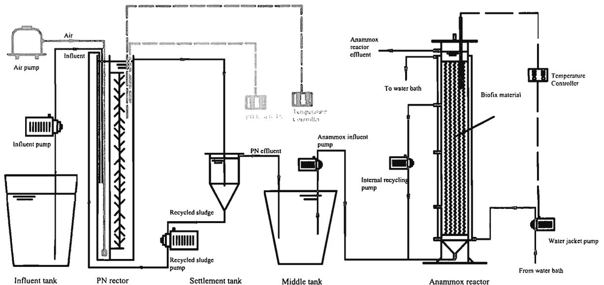
Fig. 4- 1 Schematic diagram for PN-Anammox apparatus
