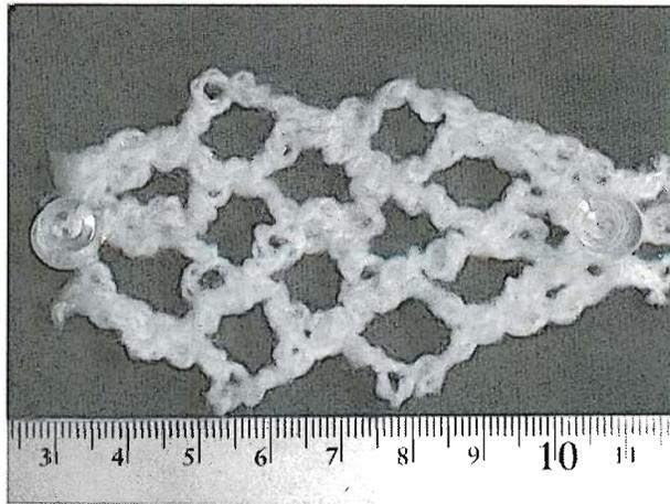
Fig. 2- 2 Photo of the acrylic fiber biomass carrier (Biofill)
