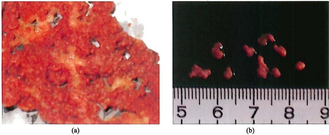
Fig. 2- 8 Anammox sludge immobilized on Biofill
