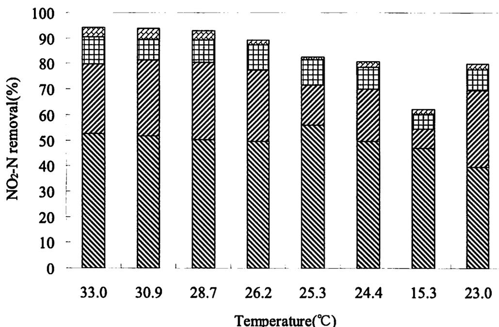
Fig. 2- 7 Effect of temperature on nitrite removal efficiencies in different height levels under NLR of 2.0 kg-TN/m<sup>3</sup>/d
