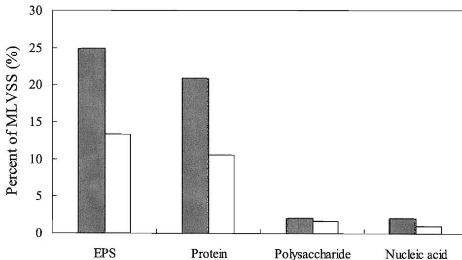
Fig. 3- 5 EPS comparison of granular and attached biomass in Biofix reactor
