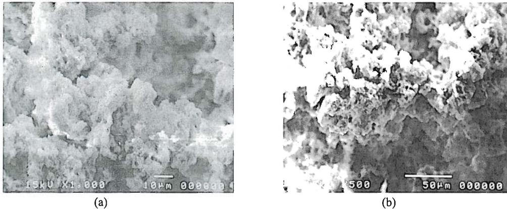
Fig. 4- 9 SEM observation of attached biomass
