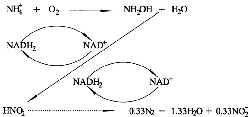
Fig. 1- 6 Independent model of nitrification and denitrification process
