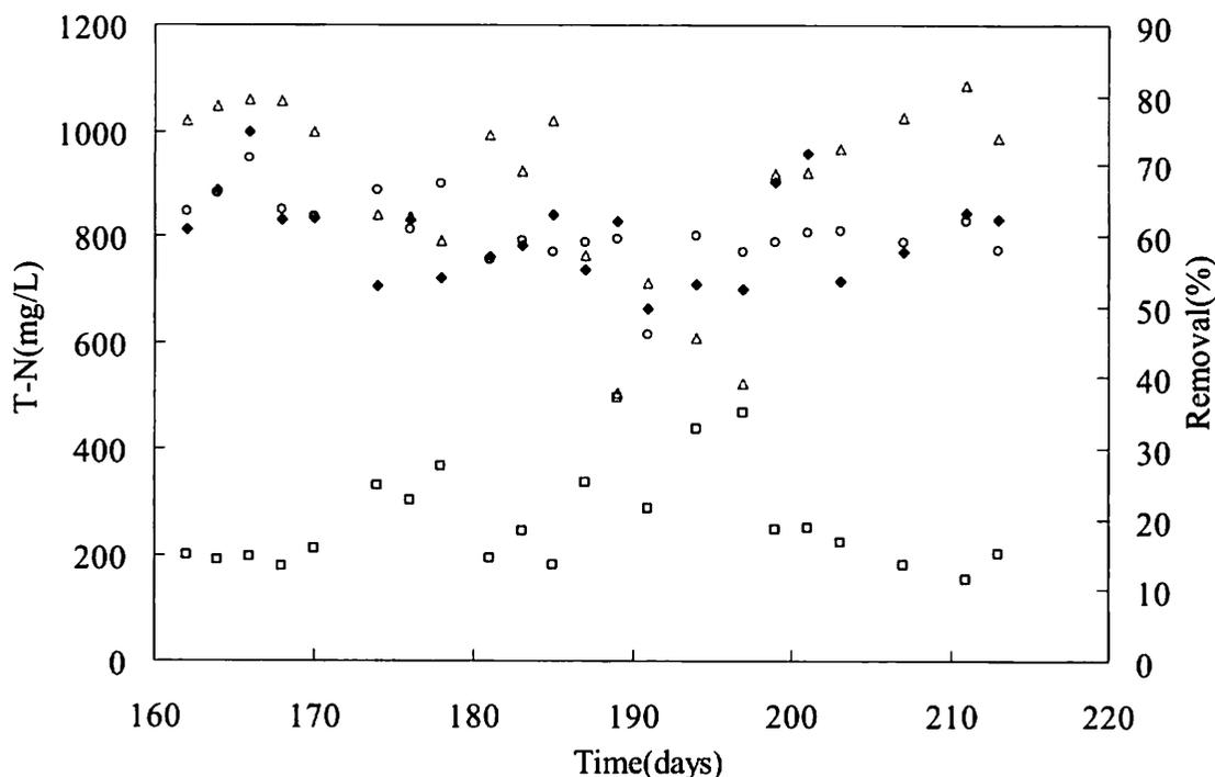
Fig. 4- 6 Time courses of T-N concentrations and removals in PN and Anammox reactor
