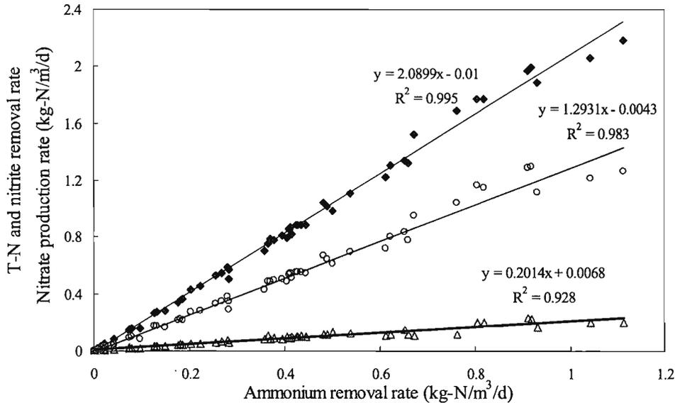
Fig. 3- 3 T-N and nitrite removals and nitrate production as functions of ammonium removals
