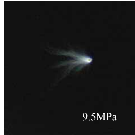
Figure 5. Photograph of the streamer discharge plasma at pressure of 9.5 \text{ MPa} and at temperature of 37 \text{ a} .
