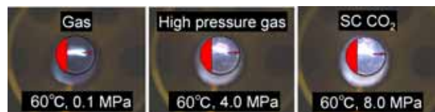
Figure 1. Pressure dependency of arc discharge in CO 2
