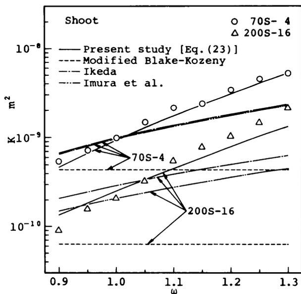
Fig. 11 Relation between permeability and packing number
