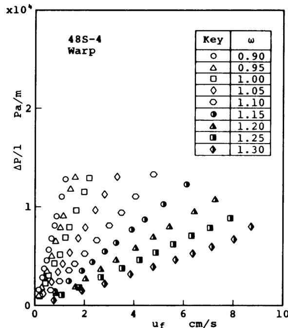
Fig. 4 Influence of packing number on pressure drop
