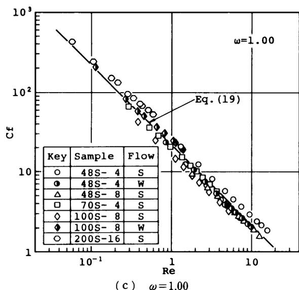
Fig. 8 Relation between friction factor and Reynolds number
