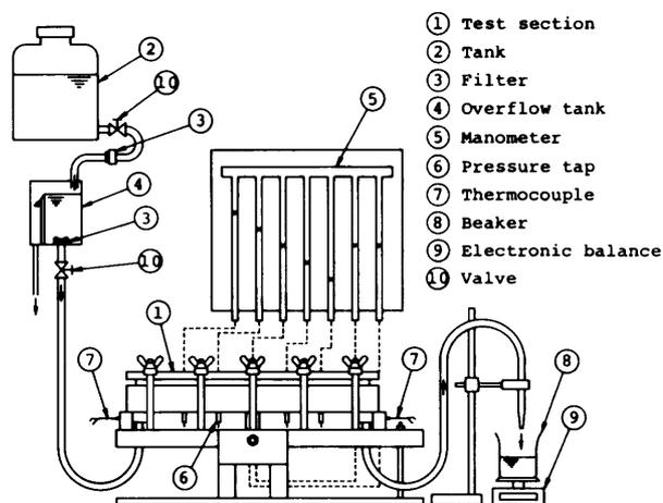
Fig. 2 Schematic diagram of apparatus for measurement of friction factor
