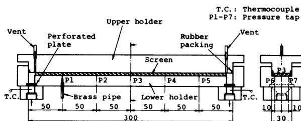
Fig. 3 Details of test section
