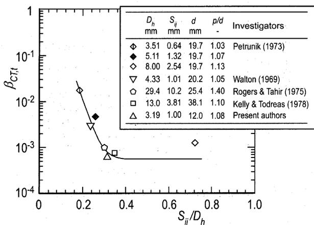
Fig. 6 Mixing Stanton number due to convective transfer for fully developed turbulent flow region in several triangle lattice channels
