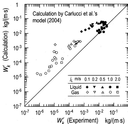
Fig. 14 Comparison of two-phase turbulent mixing rates between the present experiment and the calculation by Carlucci et al.'s model<sup>(24)</sup>
