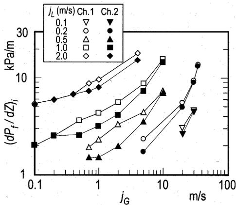
Fig. 6 Frictional pressure drop data in each subchannel
