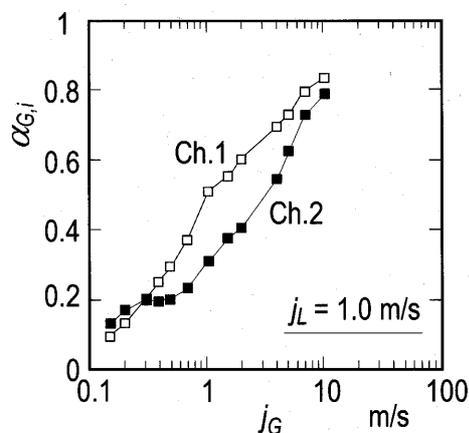
Fig. 4 Void fraction data in each subchannel at  $j_L = 1.0$  m/s
