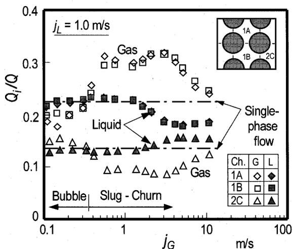
Fig. 3 Flow distribution data in a hydraulically equilibrium two-phase flow at  $j_L = 1.0$  m/s<sup>(5)</sup>
