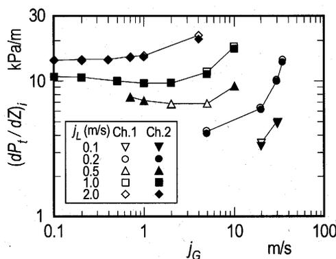
Fig. 5 Total pressure drop data in each subchannel
