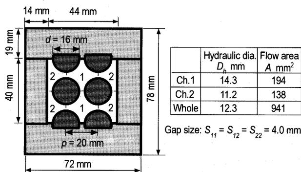
Fig. 1 Cross-section of the test channel with 2 × 3 rods
