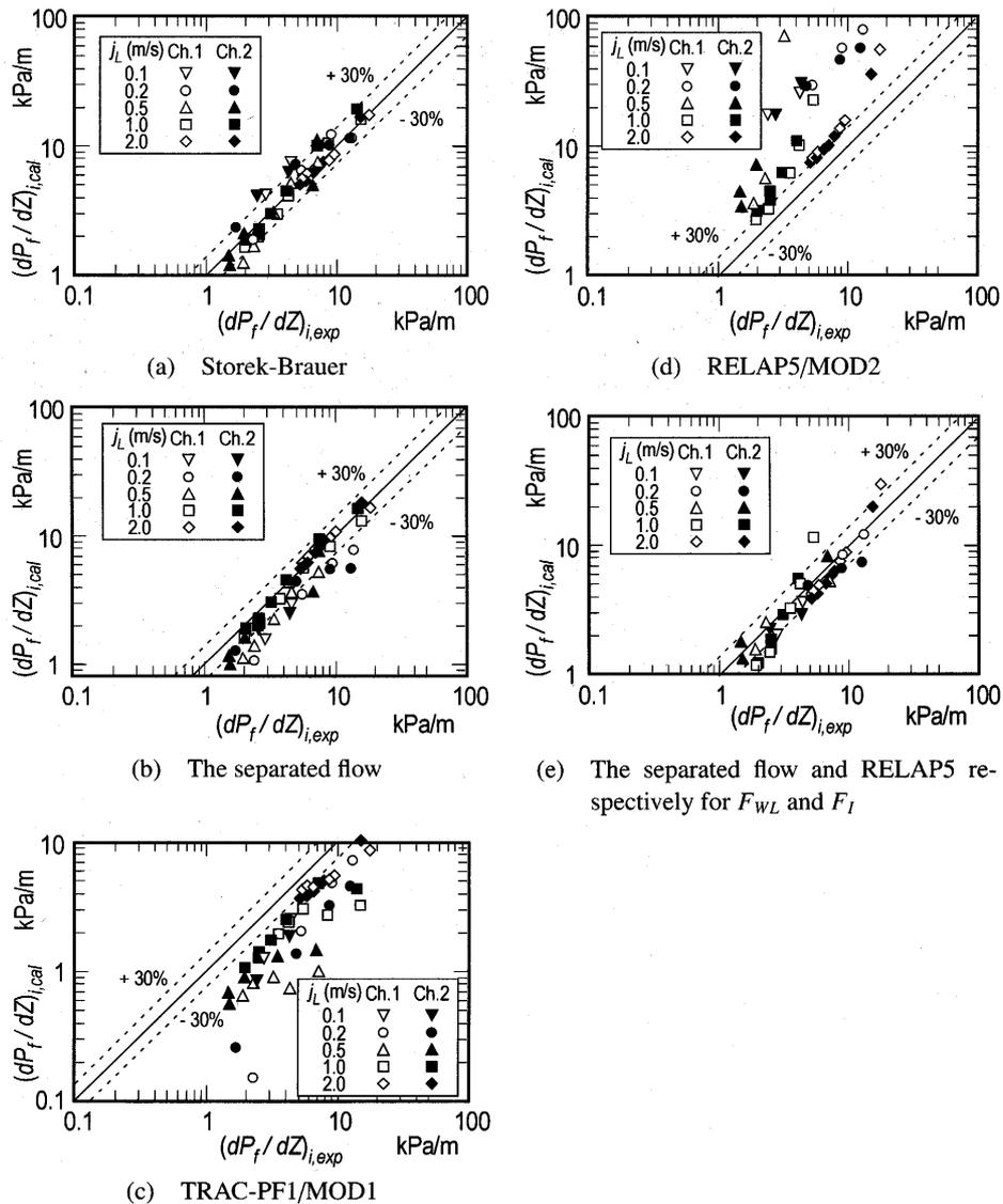
Fig. 8 Assessment of frictional pressure drop prediction
