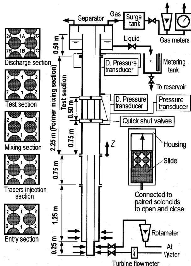
Fig. 2 Flow loop of the test channel with 2 × 3 rods
