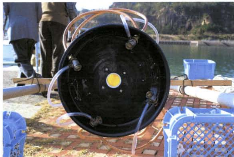
(b) Four bubble jet generators at the riser skirt
