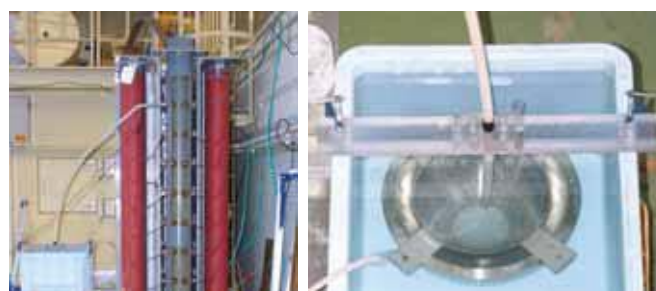
Marx generator Capacitor: 0.8 \mu\text{F} -10 stages Output voltage: 400 kV Stored energy: 6.4 kJ/shot Discharge electrodes Point to hemisphere
