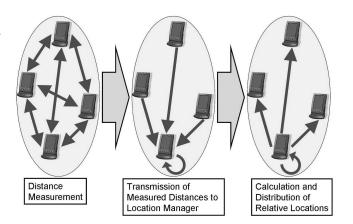
Fig. 3. Procedure for estimating relative locations.
