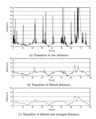
Fig. 9. Effect of noise reduction for measured distances.
