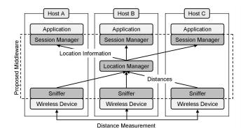
Fig. 2. Software architecture of the proposed middleware.
