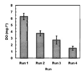
Fig. 9 DO levels in the SB reactor in different runs: bars indicate standard deviation.
