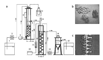
Fig. 1 (a) Schematic of the AF-SB system: (1) influent tank; (2) influent pump; (3) AF recycle pump; (4) BL carriers; (5) AF reactor; (6) thermostat heating device in AF reactor; (7) gas-liquid separator; (8) thermostat heater in SB reactor; (9) SB reactor; (10) BF carrier; (11) air flow meter; (12) air pump; (13) sludge return pump; (14) settling tank; (15) effluent tank; (b) photograph of BL carriers; (c) photograph of BF carrier.
