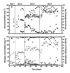
Fig. 4 (a) Changes in TN removal performance: (★) TN removal efficiency; (◊) influent TN concentration; (�) AF effluent TN concentration;
