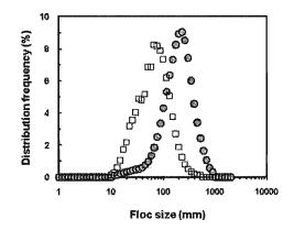
Fig. 7 Floc size distribution of sludge in the SB reactor: (□) Seed sludge, mean size: 76 µm; (●) Run 4, day 149, mean size: 213 µm.
