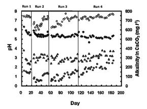
Fig. 2 Profiles of pH and alkalinity in AF and final effluents: (♠) AF effluent pH; (○) final effluent pH; (△) AF effluent alkalinity; (③) final effluent alkalinity.
