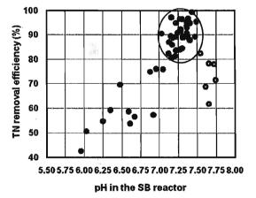
Fig. 10 Relationship between pH in the SB reactor and TN removal: (●) results in normal operation; (○) results in mechanical troubles or sludge washout.
