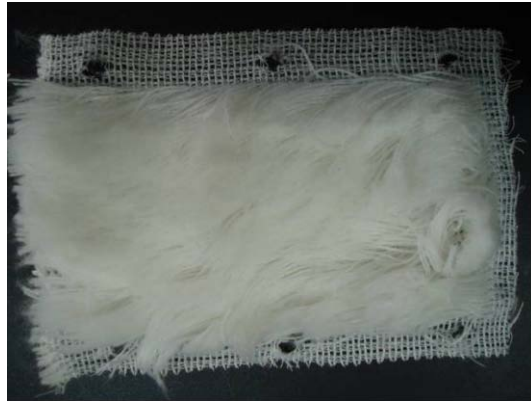
Fig. 5-3 Photographs of acrylic pile fabrics (Pile-H-36) biomass carriers material; acrylic fiber diameter of a pile; 1 mm length of pile; 3 cm
