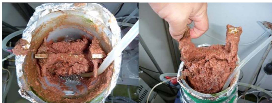
Fig. 5-15 Photographs of biomass carriers (Pile-H-36) at days 809 of SNAP treatment
