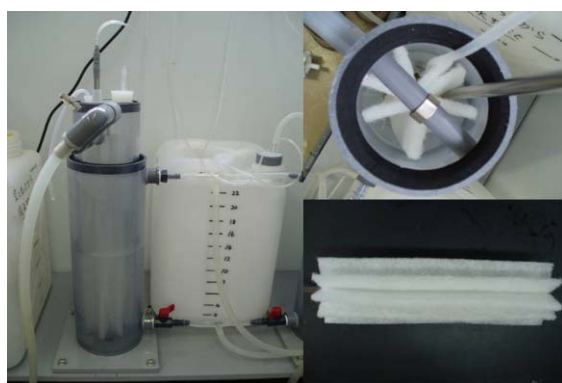
Fig. 5-1 Photographs of up-flow ANAMMOX column reactor and non-woven as biomass carrier
