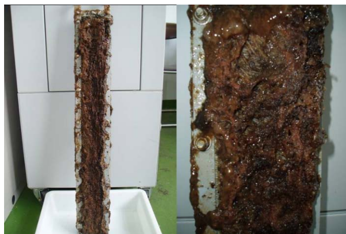
Fig. 5-10 Photographs of biomass carriers (Pile-H-36) at days 434 in SNAP treatment
