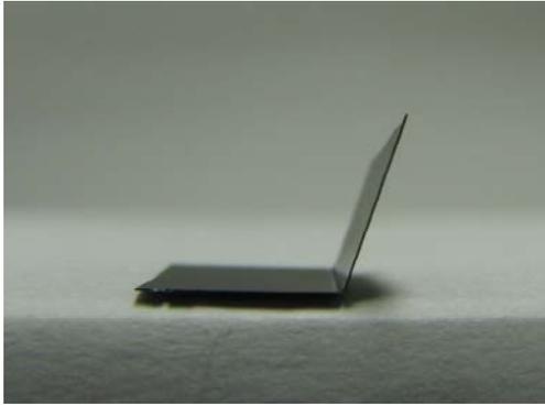
Bent single crystalline silicon
