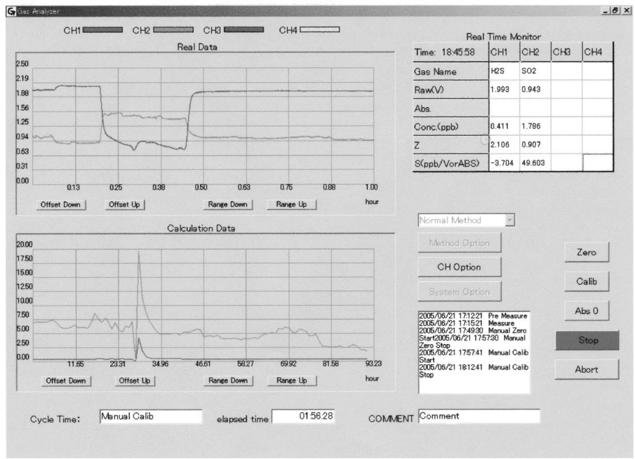
Fig. 2 Program for system control, data acquisition and data processing Flow diagram (above) and display in the computer screen (below)
