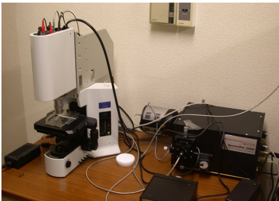
Fig. 2.15 Photograph of micro-Raman measurement system.
