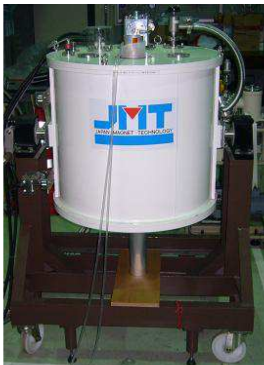
Fig. 2.24 Photograph of the 10 T cryocooler-cooled superconducting magnet used in this study.
