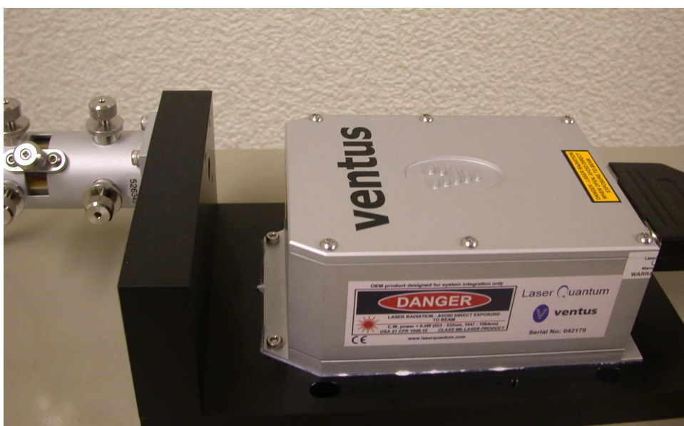
Fig. 2.16 Photograph of semiconductor laser of the micro-Raman measurement system.
