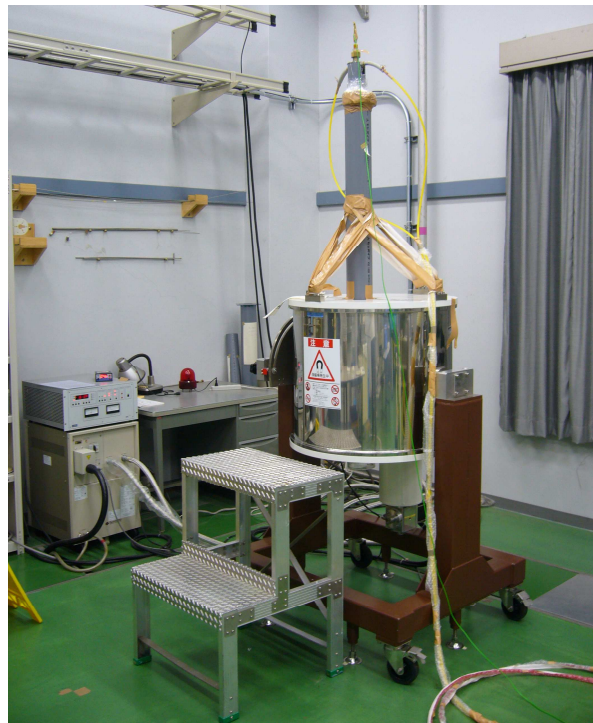
Fig. 2.23 Photograph of the 12 T cryocooler-cooled superconducting magnet used in this study.
