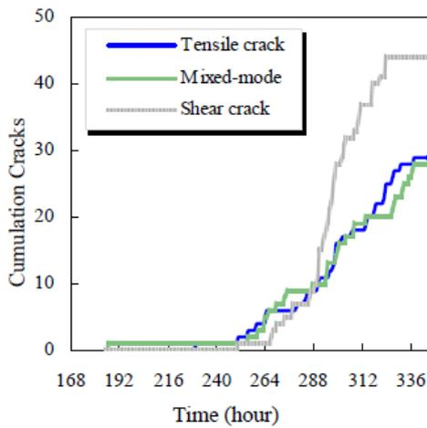
Figure 21. Cumulation Cracks of classify crack type.
