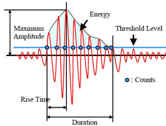
Figure 3. AE signal parameters.
