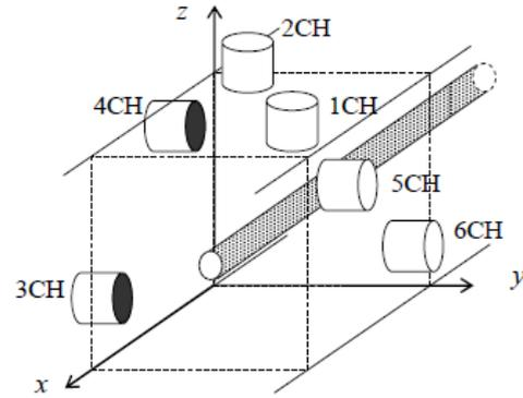
Figure 11. Set of AE sensors.
