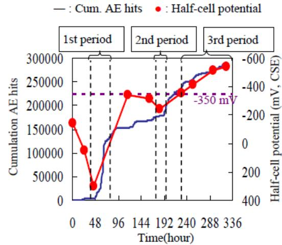
Figure 14. Cumulation AE hits and Half-cell potentials
