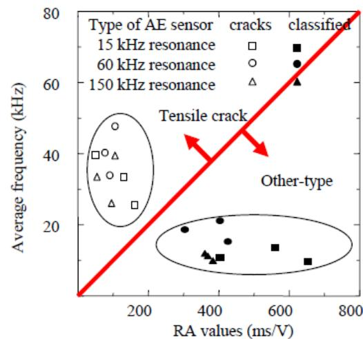
Figure 4. Classification of cracks by AE indices.
