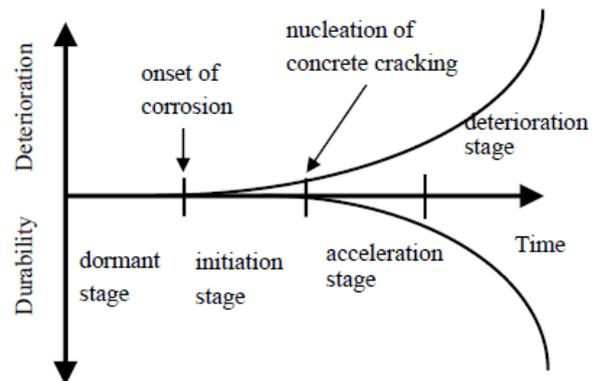
Figure 1. Deterioration process due to corrosion.
