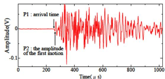
Figure 5. Detected AE waveform.
