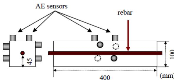
Figure 9. Sketch of Reinforced concrete slab tested.
