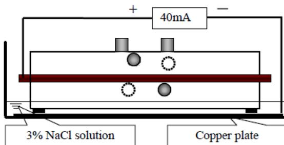
Figure 10. Test set up for accelerated corrosion test.
