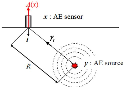
Figure 6. Crack nucleation and AE detection.
