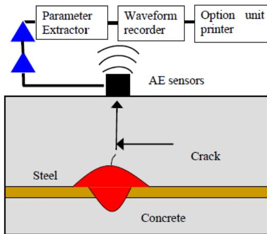
Figure 2. AE measurement.
