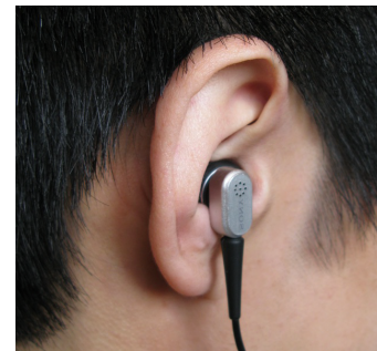
Fig. 2. Canal type actuator and combined sensor used for an implementation of binaural hearing assistance system whose directivity pattern is shown Fig.1.
