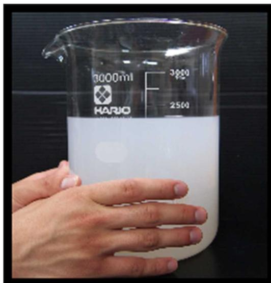
**Figure 3-5. Photograph of the mass-product DS nanosheet solution (2L,  $3.9 \times 10^{-3} \text{M}$ ).**
