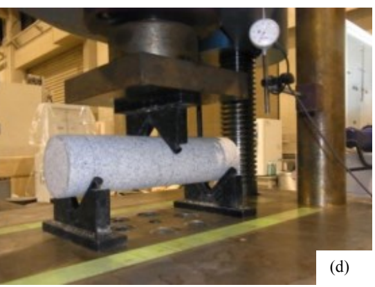
Fig.11 Specimens, loading jig and view of TPBr test : (a) beam having a rectangular cross section; (b) beam having a circular cross section; (c) loading jig; (d) view of three-point bending test for the specimen having a circular cross section.
