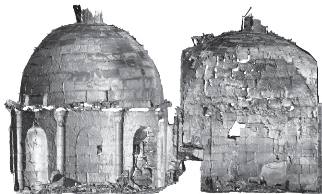
Fig. 5 Petra, point-cloud image of the Baths, section looking from the west to the east
