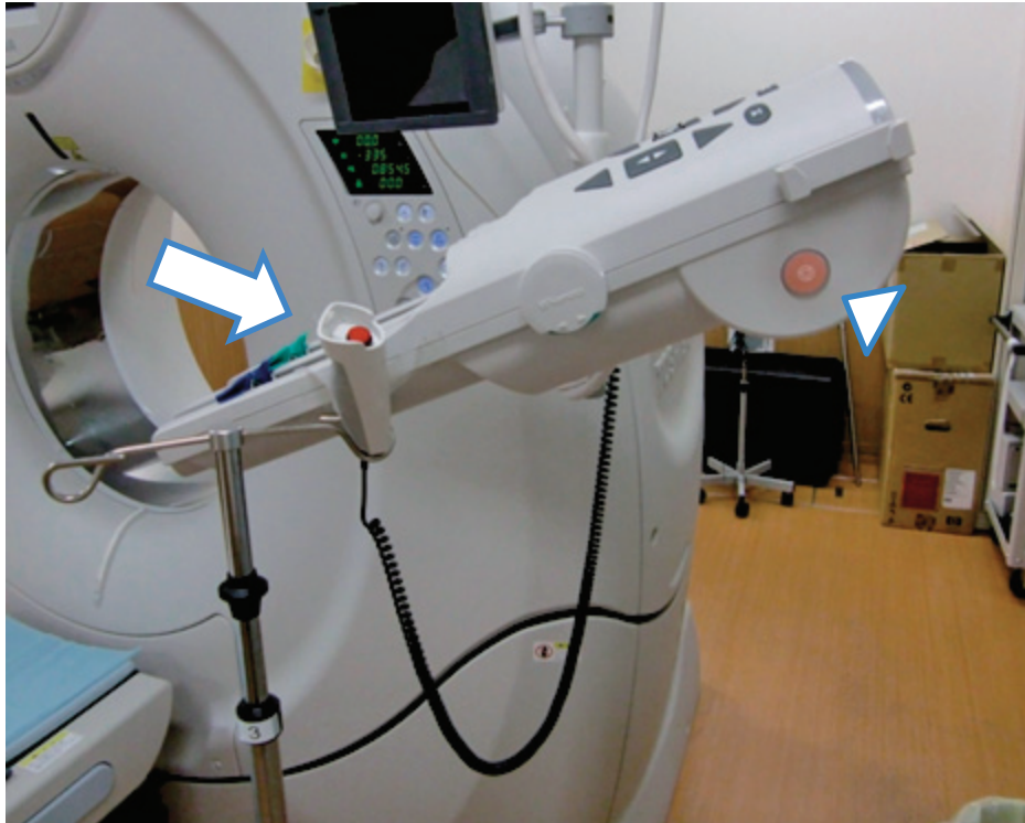
Fig. 3.6 An example of countermeasure for one incident in CT examination. Before the incident occurred, only one emergency stop button (arrow head) was located on the injector. For prevention of incident, an additional emergency stop button with flexible cable (arrow) was supplied.
