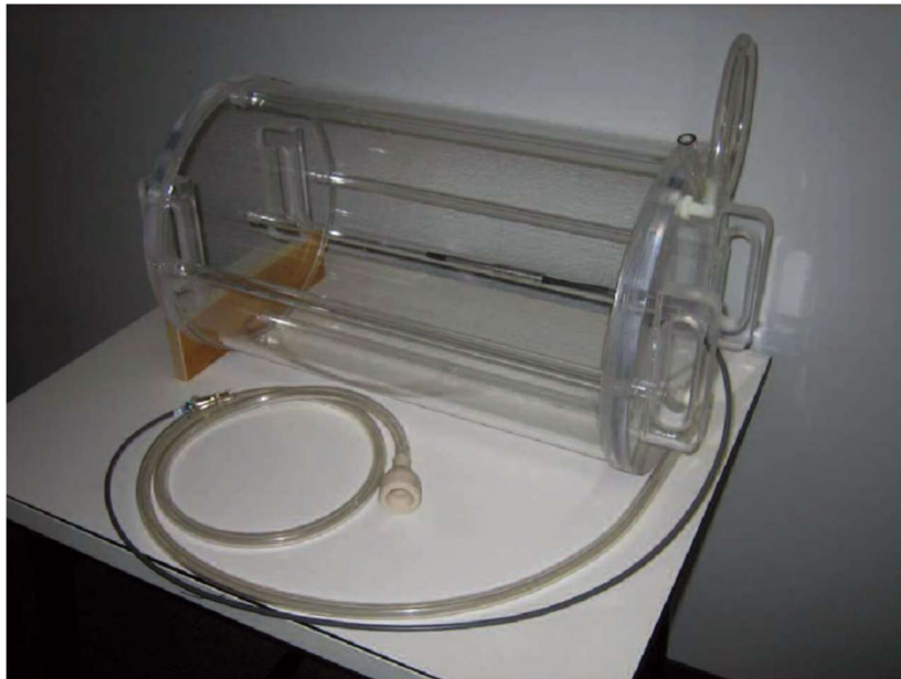
Fig. 1-11. The schematic image of cylindrical water phantom with 30 cm diameter and 50 cm length 12) .
