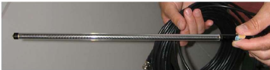
Fig. 1-9. The schematic image of 300 mm CT pencil chamber 15)
