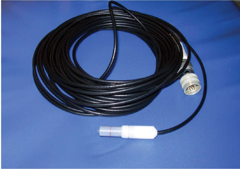
Fig. 1-12. The schematic image of Farmer chamber with 0.6 cc volume 12) .
