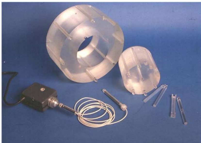
Fig. 1-4. The schematic image of CTDI phantom and 100 mm CT pencil chamber 12) .
