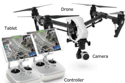
Fig.3 Drone used in this study. (revise figure in http://www.sekido-rc.com/ )
