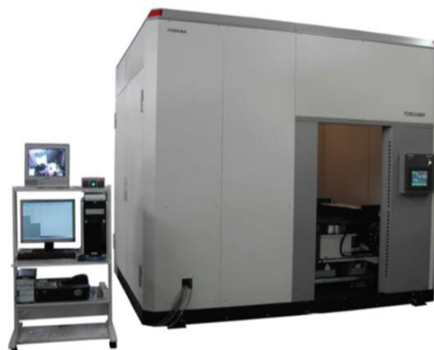
Fig. 7. Outlook of industrial use X-Ray CT scanner operated by Kumamoto University (TOSCANNER-20000RE).
