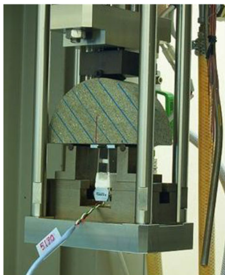
Fig. 3 SCB specimen loading fixture
