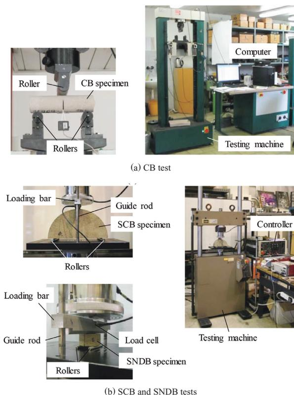
Fig.3 Setup of specimen with loading apparatus placed on testing machine<sup>20)</sup>.
