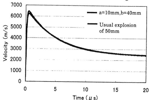
Figure 3. Velocity histories of underwater shock wave in the case of total length of 50mm
