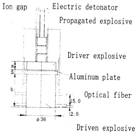
Figure 1. Experimental device
