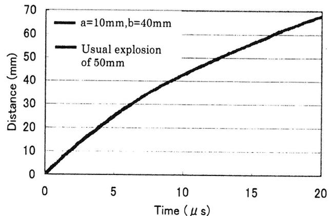
Figure 2. Inclination diagram of underwater shock wave in the case of total length of 20mm
