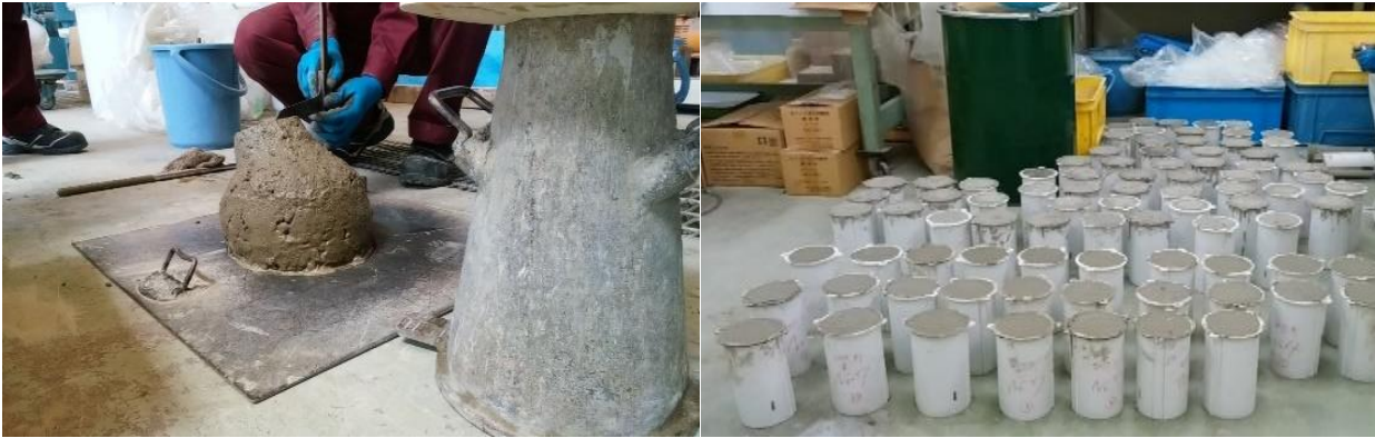
Figure 7.3 Slump test and samples after casting in molds
