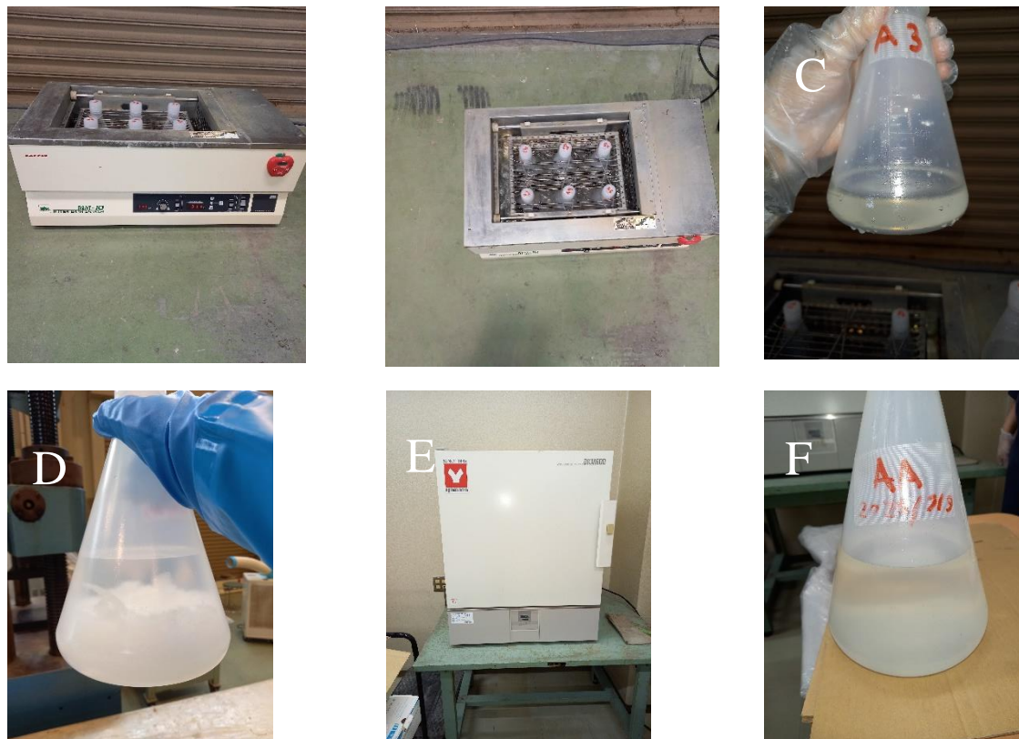
Figure 5.1. Making alkaline solution: (A, B) Water Bath Shaker, (C) AA solution after dissolution process, (D) Crystallization of the solutes, (E) An incubator, (F) AA solution after heat treatment in the incubator.
